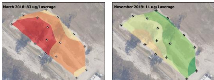
Montrose Regenerable Resin Solution Before & After PFAS Plume
